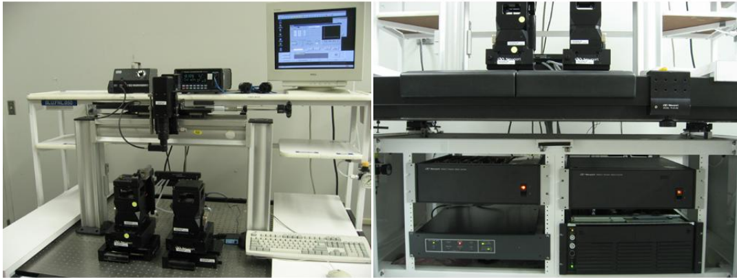
Top View (L) with stages, camera, monitor, power meter. Bottom View (R) with computer, controllers and UPS.
